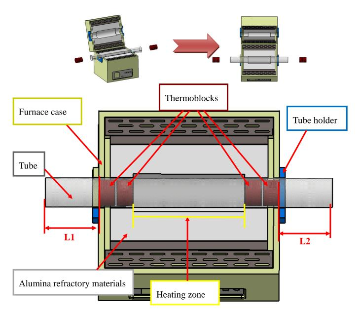
Our high temperature OTF series (for  $1500\,\mathrm{C}$  grade and up) furnaces require two thermoblocks on each side.
